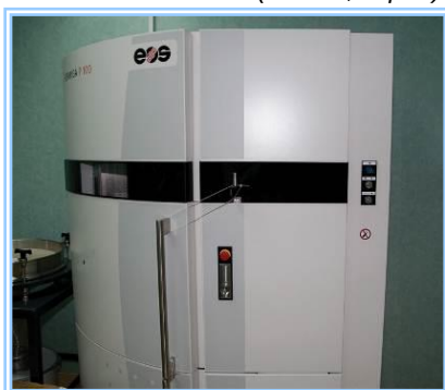
3D Printer with Selective Laser Sintering - Formiga P100 (EOS GmbH, Germany)
