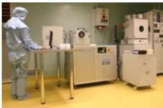
RIE Plasma Etcher - Etchlab 200 (SENTECH Instruments, Germany)
