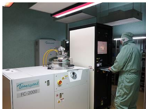
E-Beam Deposition system (Temescal, USA)
